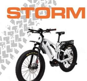
**Motor:** Bafang Ultra M620 750w/1000w Mid-Drive Motor w/Integrated Torque Sensor
